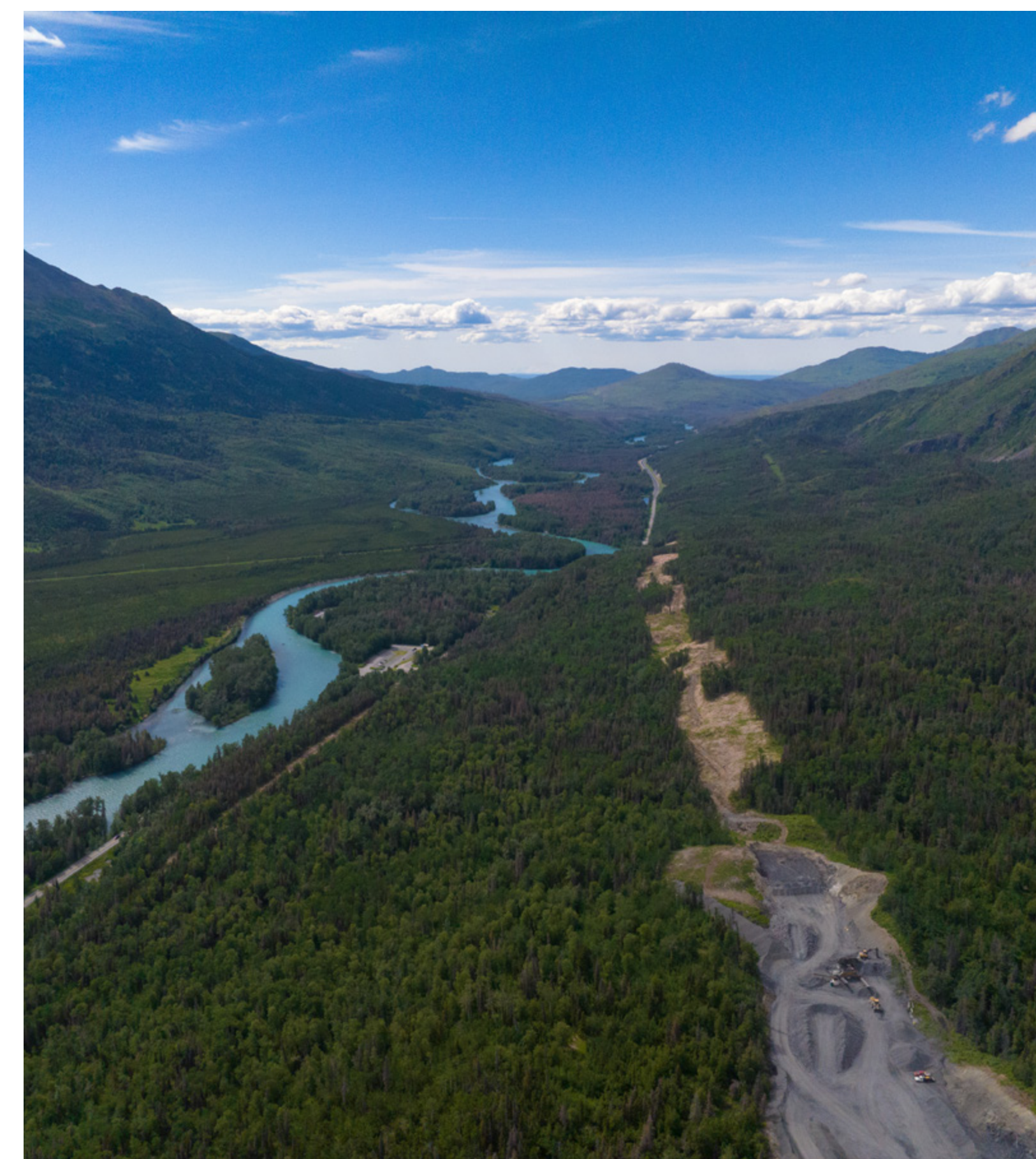
Phases 4 & 5: Transition from the Phase 4 (gravel surface) to Phase 5 (cleared area). A screening plant is setup for material production and sorting. Geological and Archeological crews working in Phase 5.
